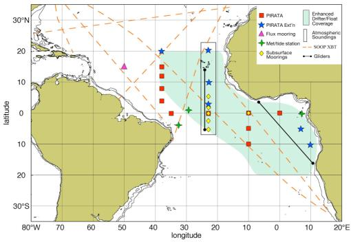
FIGURE 2. TACE Observational Strategy. The proposed observing system components include (see legend): Continuation of PIRATA moorings, PIRATA extensions along 23 ° W and 5-10° E, equatorial subsurface (non-realtime) moorings along 23 °E and at 10° W, island meteorological and tide gauge stations, enhanced float/drifter coverage in the eastern TA, repeated atmospheric soundings along 23 °W, ship-of-opportunity XBT lines, and selected glider transects (see the "TACE Synopsis" for more details).
