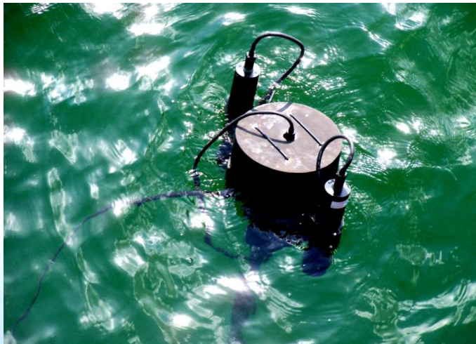
Hyperspectral radiometer deployed during a Noctiluca Scintillans bloom in the northern Arabian Sea.
